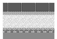
Concrete paving Bedding material
